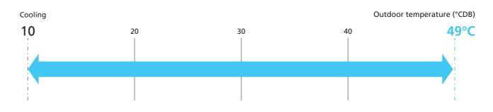
Note: When outdoor temperature falls below 10℃, the thermostat shuts OFF, the outdoor unit stops, and operation switches from cooling to fan operation.
